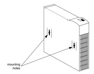
These slots fit over the heads of wall-mounting screws to secure the modem to the wall.
